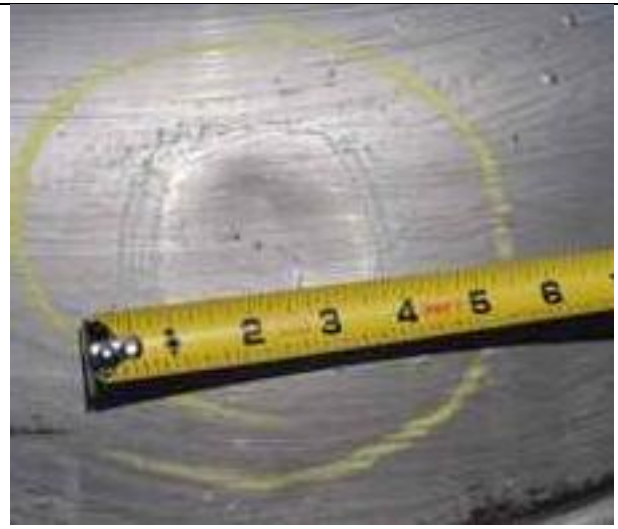
4.09-6. Large size indentation on the metal exhaust unit.
