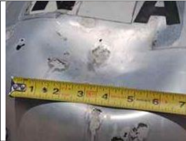
3.12-1. Large hail dent in vent stack.
