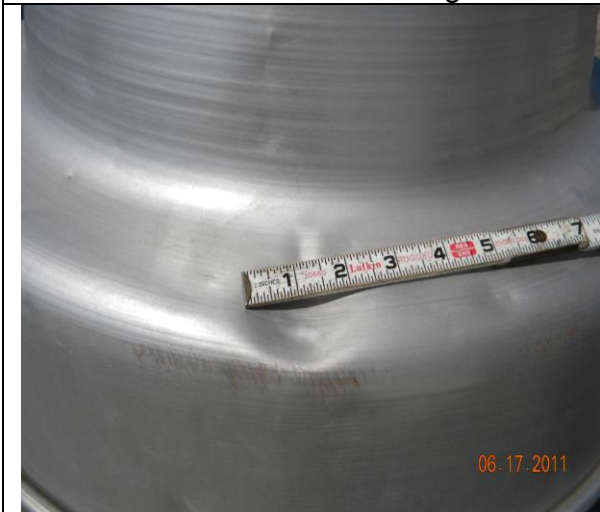
01.26-3. Close view of impact damage in vent cover ~ 1.5-inch.
