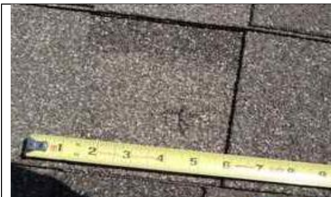
6.13-1. View of granule damage and mat fracture.
