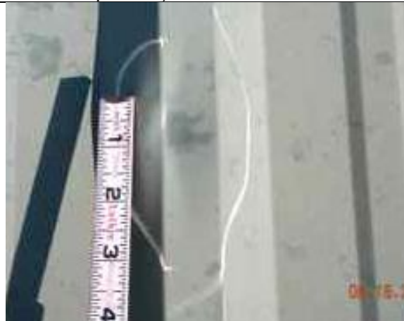
1.16-4. Close-up of impact depressions in metal roof rib in Photo 3.
