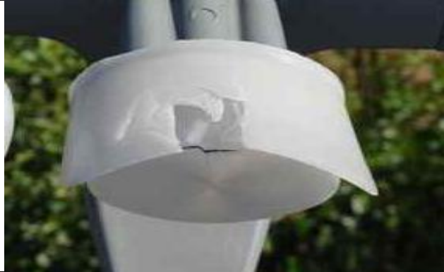
5.10-7. Broken plastic receiver on satellite dish
