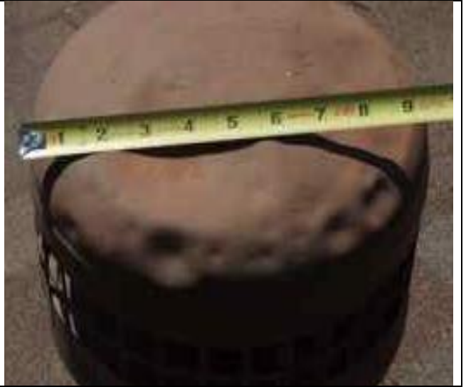
6.11-2. Dents in aluminum vent cap.
