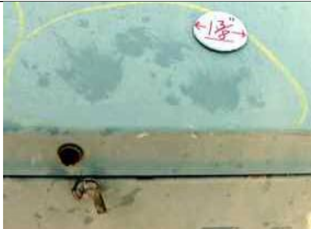
4.06-3. Spatter marks on the top surface of the AC unit.
