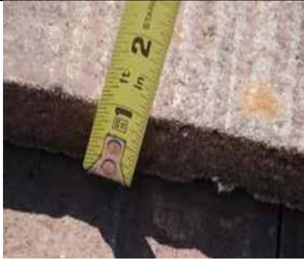
3.11-1. Thickness of concrete tile.
