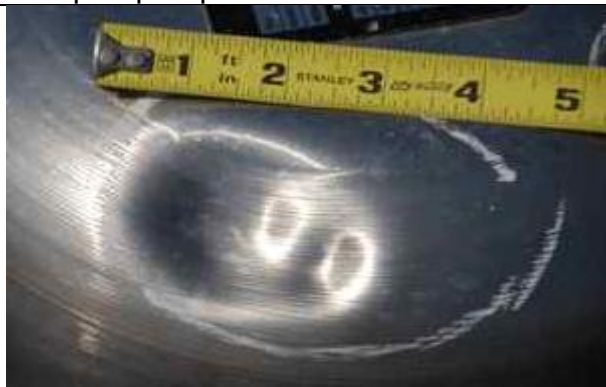
3.09-3. Large dent in exhaust fan from hail impact.
