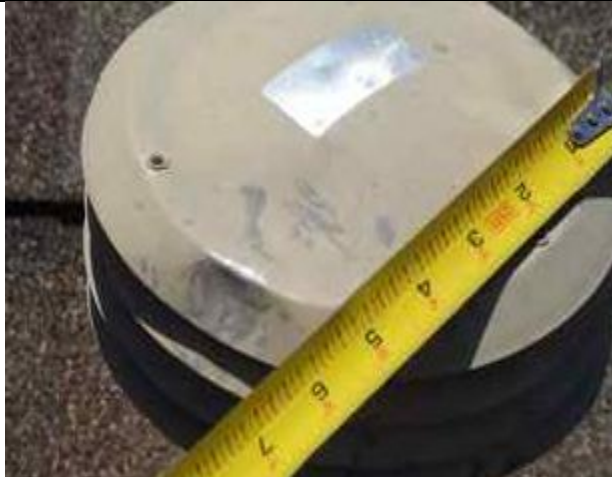
5.18-5. Dent and spatter mark on metal vents
