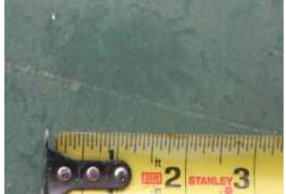
2.19-10. Two-inch wide spatter mark on transformer box.
