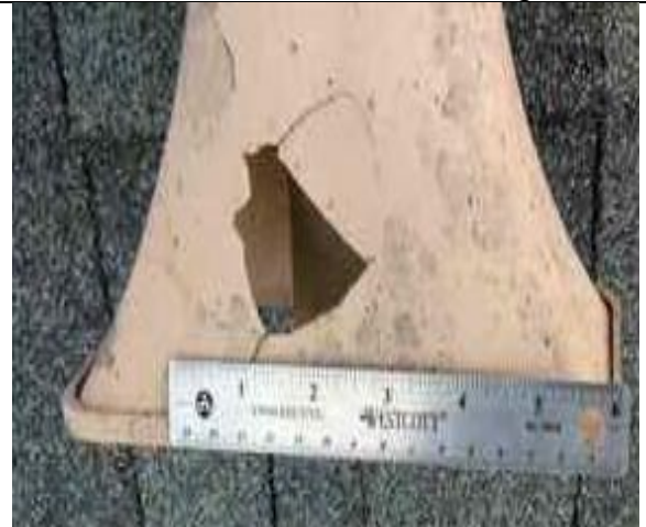
4.05-4. Punctured plastic equipment on the roof.
