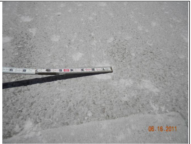
01-20.6. Hail bruising marks on roof top unit.
