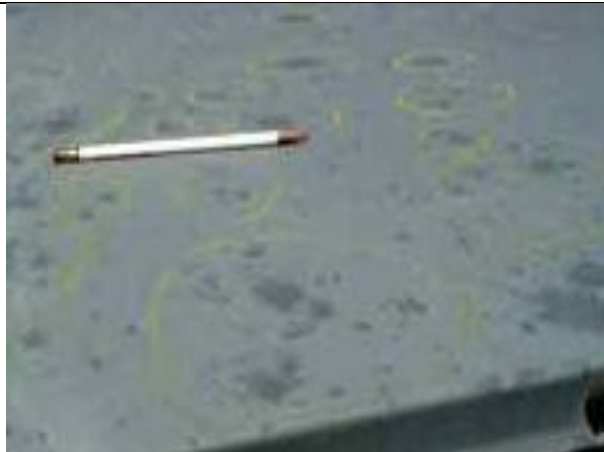
4.06-7. Several spatter marks on the top surface of the AC unit.
