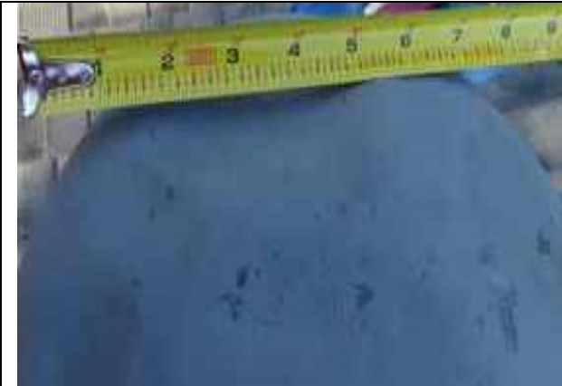
5.13-1. Dents and splatter marks in metal vent.
