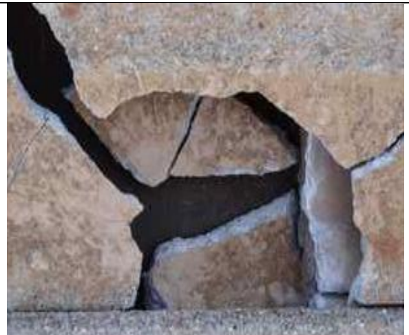
5.16-4. Close up of fracture from large hail impact, with splatter mark.
