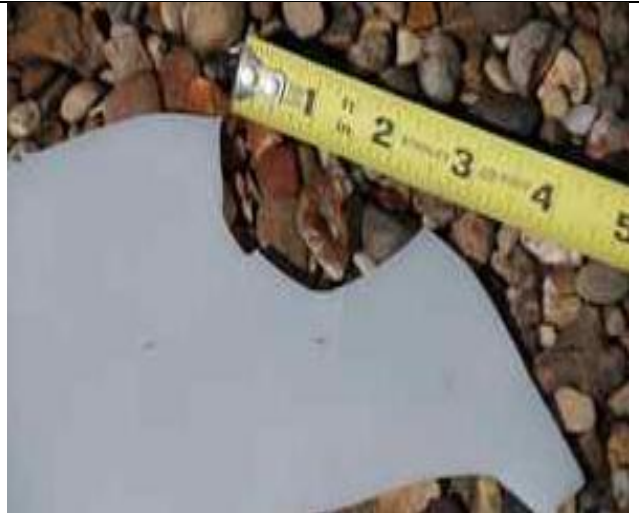
3.10-2. Sample of broken skylight due to hail impact.
