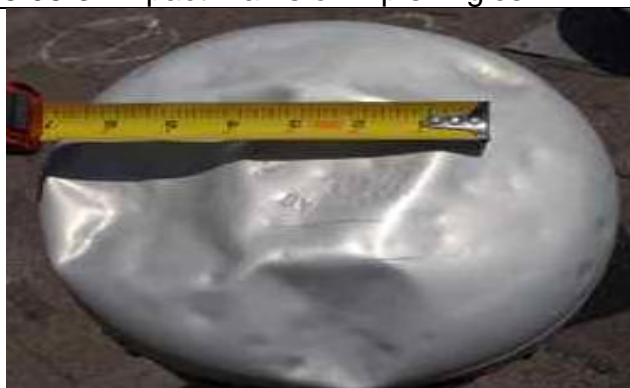
5.06-5. Impact marks on metal vent cover.
