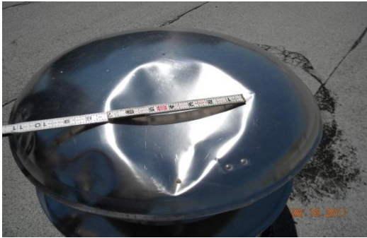
Figure 1. Vent cap buckled by large hail in Irving.
