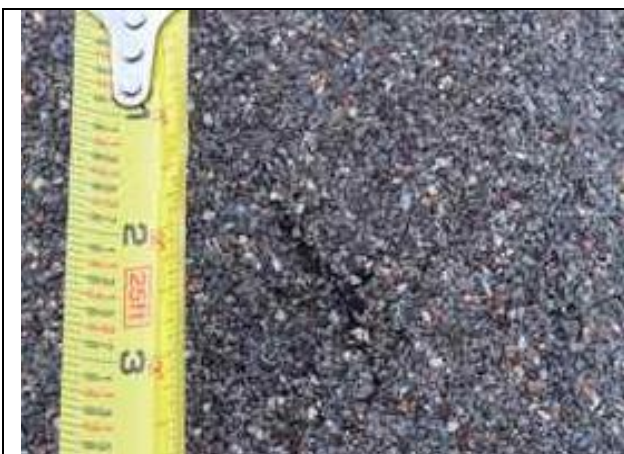
5.18-1. Fracture in asphalt shingle.
