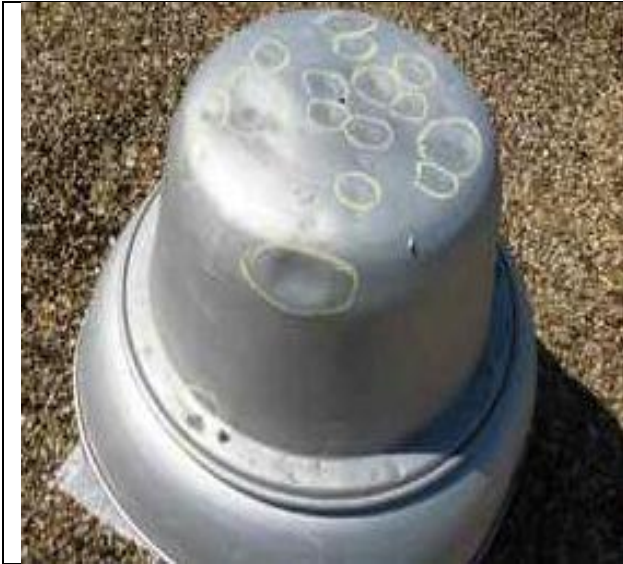
4.09-1. This exhaust unit was hit by numerous hailstones of moderate to large size.
