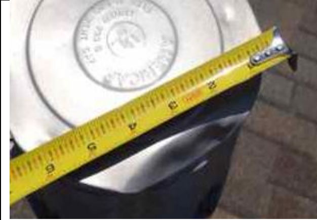
5.18-7. Large dent on edge of metal vent.
