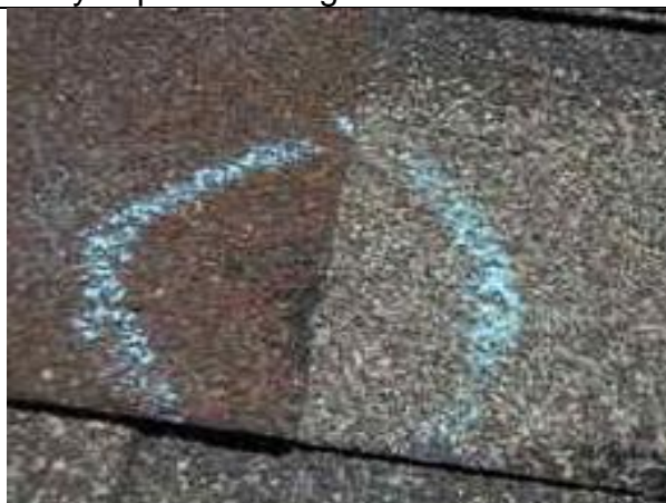
1.11-3. Close-up of "bruised" shingle laminate.
