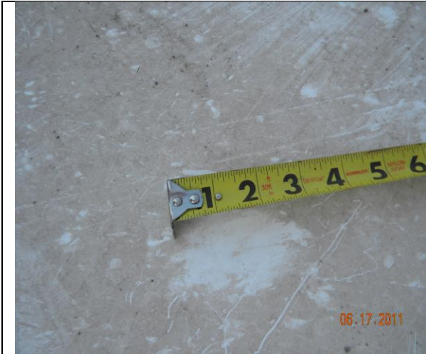
01.26-1. Close view of impact marks on TPO membrane with no damage.
