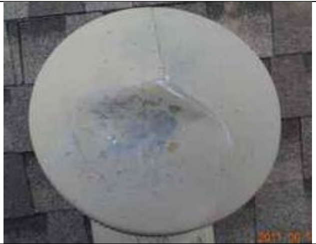
6.01-2. Dent boundary and coinciding splash mark.
