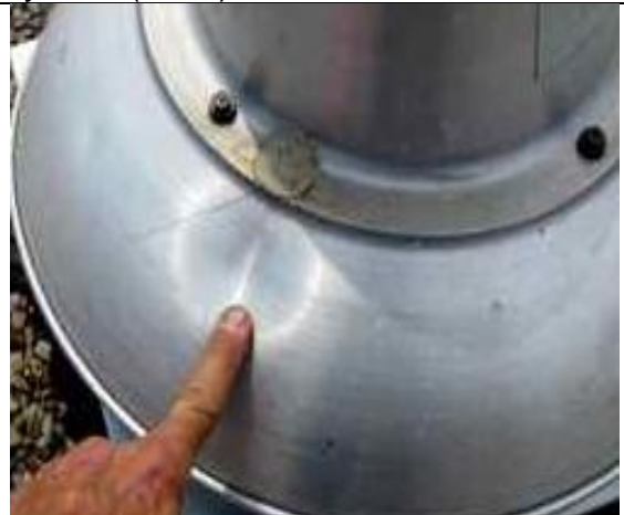
4.02-4. This indentation in an exhaust cover is approximately the size of an egg.
