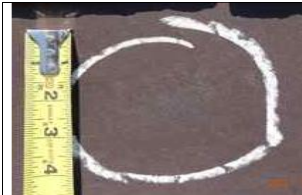
6.07-1. Splash mark on synthetic simulated slate.
